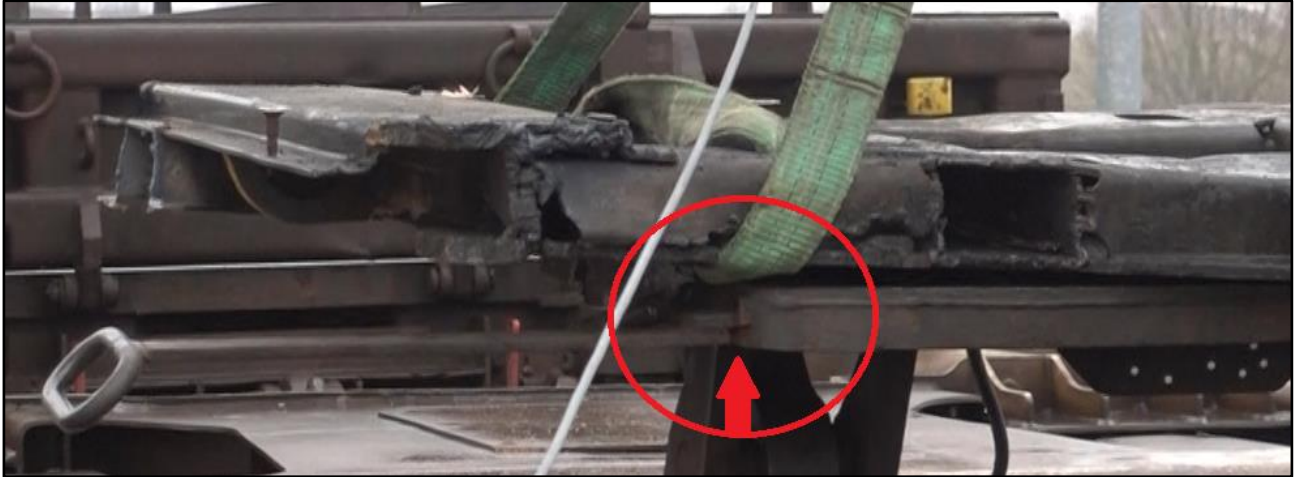
Figure 2. Operating handle position after king pin has been lowered into the hitch. Gap is 8,66 mm.
